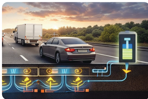
Figure 6. Road-embedded piezoelectric energy harvesting concept.
